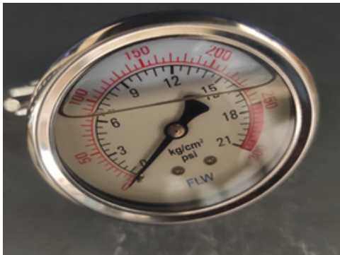
PRESSURE GAUGE FOR WATER PRESSURE Minimum inlet water pressure should be 0.5bar
