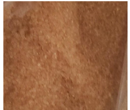
RESIN FOR REMOVAL OF HARDNESS It removes the hardness from the water which is in the form of Calcium and magnesium
