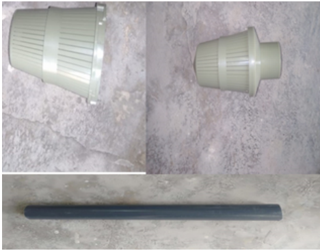
TOP AND BOTTOM STAINER WITH PIPE To restrict resin beads passing through the water
